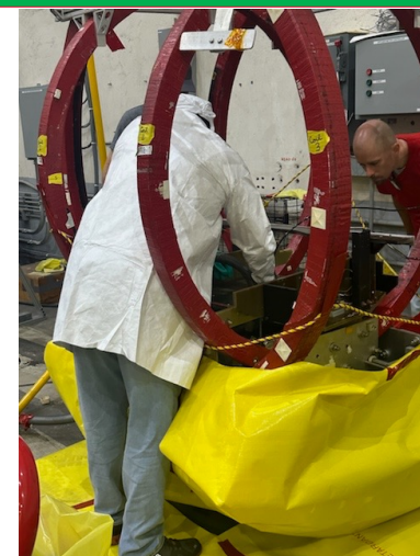
Fig 5. Helmholtz coils are used to induce the magnetic field. The coils were contaminated in the previous set-up, so we and RadCon cleaned them. This meant we all had to receive RadWorker II training.
